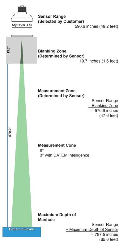
**Maximum Depth of Sensor** is calculated using the 16.4 ft cable length and estimated mounting of the MyLevel device and sensor near the top of the manhole
